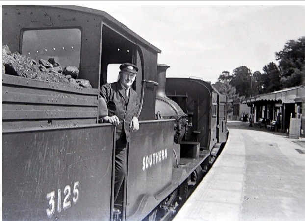
Image 1: Taken between 1940 and 1948. Percy on the footplate of the Adams Radial Tank that was ultimately re-numbered 30582. The livery is the Southern Railway wartime black introduced to make engines look cleaner when there was little time to clean them. This was one of a trio of Adams Radial locos collectively known as 'Lyme Billy' - it was built in 1885 and ran on the line from 1913 until 1961.
