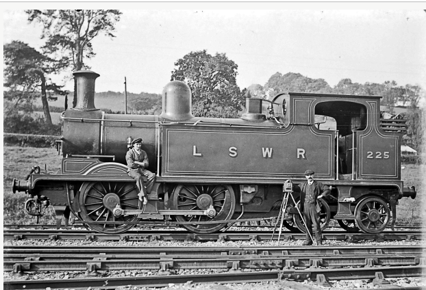
Image 2: We think the young man seated on the loco is Percy Bird, so in this case he wasn't the photographer. The photo goes all the way back to 1906 - 13 when the London & South West Railway ran O2 0-4-4 tank engines on the Lyme Regis line. They were too heavy, so ran with half-full water tanks to lighten them, but still suffered extensive damage from the tight curves. The problem was solved in 1913 with the arrival of the Adams Radial engine.
